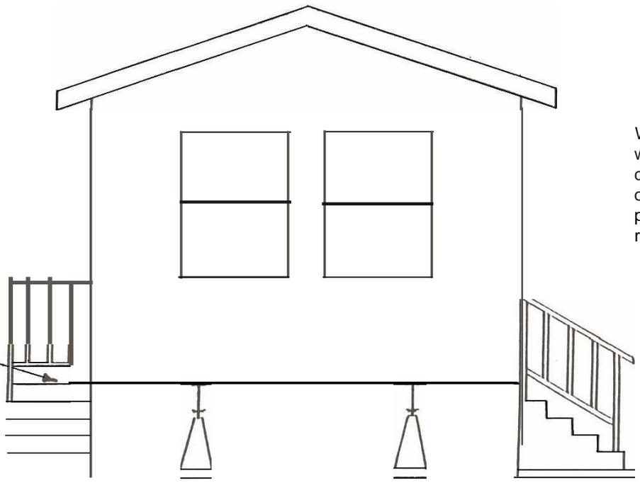
When stairways constructed of wood are placed directly on concrete or are within 6 inches of earth, the wood shall be pressure treated or of natural resistance to decay.
