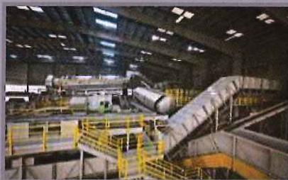
The recyclables will be processed at CR&R's Material Recovery Facility (MRF). The recyclables are separated utilizing a process of manual and mechanical sorting. These combined processes ensure that the maximum amount of recyclables are recovered from the waste stream and kept out of the landfill.
